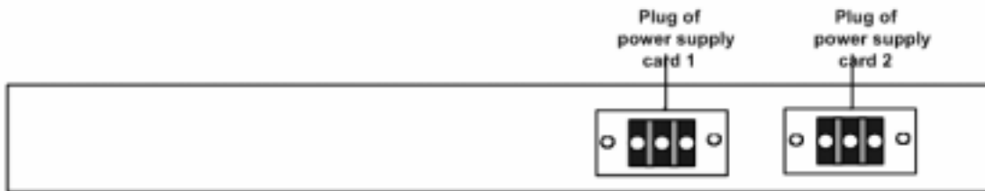
Figure 4-6 RC701/702-FE rear view of DC power supply
