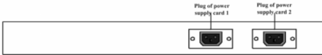
Figure 4-5 RC701/702-FE rear view of AC power supply
